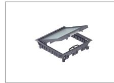
Service outlet for nine accessories in three GB3 mounting boxes for use in trunking systems and raised floors. Universal fixing bracket, adjustable to raised floor thicknesses to 65 mm. Carpet protection frame, hinged cover and cord outlet made of polyamide.
